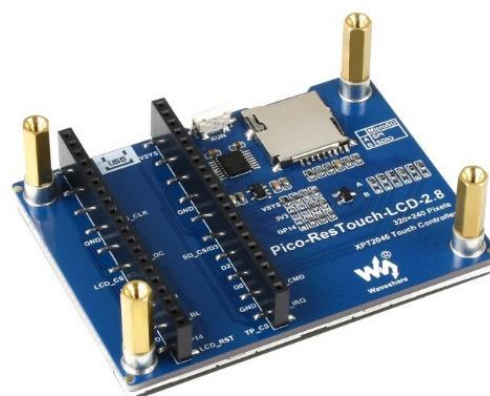
Obrázek 30 - Displej pro Raspberry Pi Pico. WAVESHARE. 2.8inch Touch Display Module for Raspberry Pi Pico, 262K Colors, 320×240, SPI. Online. Waveshare. C2025. Dostupné z: https://www.waveshare.com/pico-restouch-lcd-2.8.htm . [cit. 2025-03-21].
